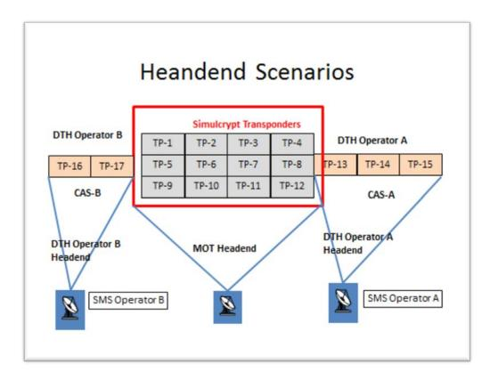
The MoT headend can transmit all the transponders which have common encryption. For the transponders which are unique to DTH operator A, the transmission can be either via the MOT, or the additional transponders can be uplinked by DTH operator A from its own headend, and likewise for DTH operator B.
