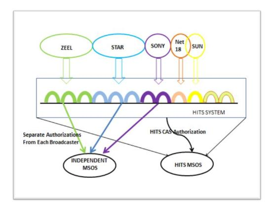
The advantage of the HITS system in this case is retained as the MSOs still require only a small antenna and Trans-Mux units as is the case for the normal HITS. Only they will have five-six decoders which will get authorized by either HITS operator (if they are parented to HITS) or by each broadcaster, if they are "independent MSOs".
