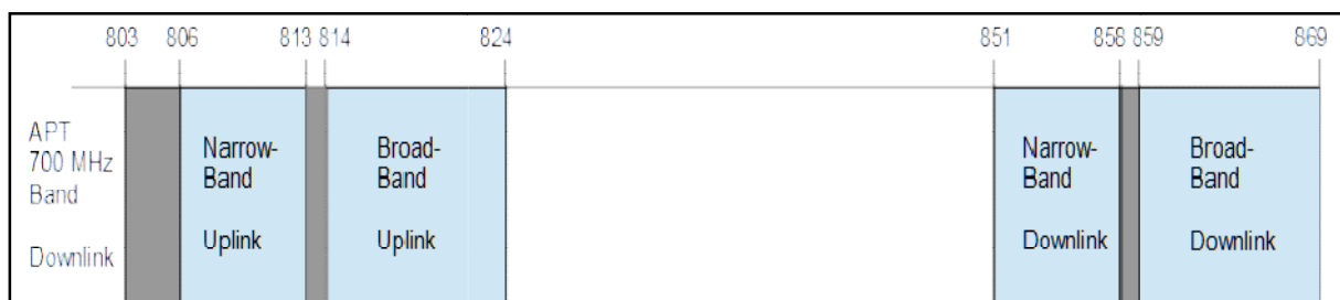
Figure 3.1: Example of frequency arrangement for a combination of narrowband and broadband systems
